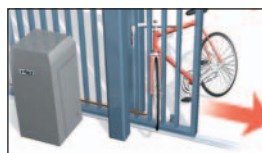
entrapment prevention system reverses gate on contact
