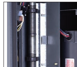
limit switches direct driven and easily adjustable
