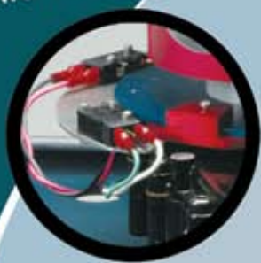
Simple limit switch arrangement
