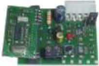
ONE-CHANNEL SELF-LEARNING SUPERHETERODYNE ROLLING CODE RECEIVER 10 USERS PLUG-IN
