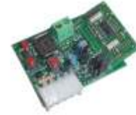
TWO-CHANNEL SELF-LEARNING SUPERHETERODYNE ROLLING CODE RECEIVER 50 USERS PLUG-IN
