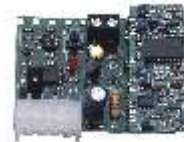
TWO-CHANNEL SELF-LEARNING SUPERHET. RECEIVER 50 USERS PLUG-IN
