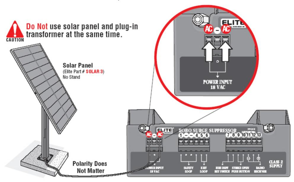
Energizing this operator with solar power only needs the radio receiver to operate the gate. The only recommended external devices other than radio receivers are dry-contact command devices which do not consume any current like key switches. Using other devices that consume high current such as telephone access, magnetic locks or loop detectors will cause excess drainage of the battery and eventually completely drain the battery.
