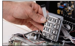
telephone access systems use a modular design concept that makes installation and service easy
