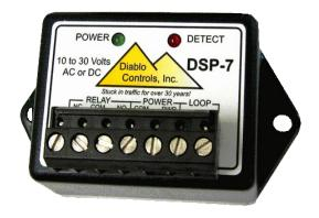
Outputs - Both N.O. (closes for detect) and N.C. (opens for detect) outputs. (1 amp max.)
