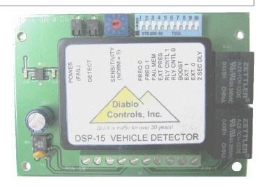
**Sensitivity** - Experience has shown that almost all parking and access control applications can be handled with sensitivity set at NORMAL (level 5). The rotary sensitivity switch is rarely moved from NORMAL. However, the DSP-15 has ten sensitivity settings varying from LOW (level 0) to HIGH (level 9).
